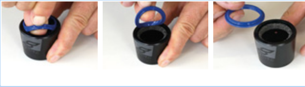
Illustration 177 : Retirer le joint anti-poussière
