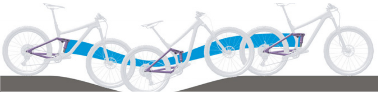
Figure 296: Excessively soft suspension in the rear frame damper on hilly terrain
