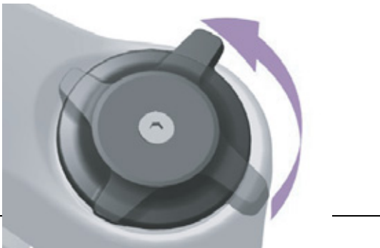
Figure 179: Changing compression adjuster to a softer setting
