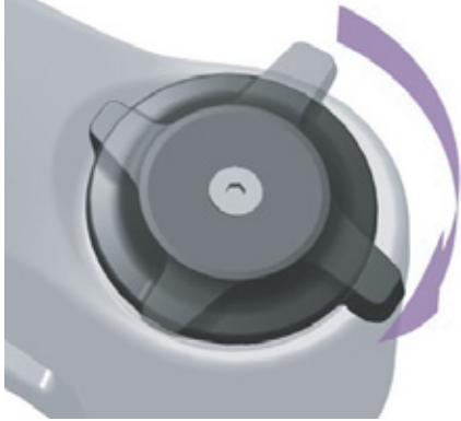
Figure 178: Changing compression adjuster to a harder setting
