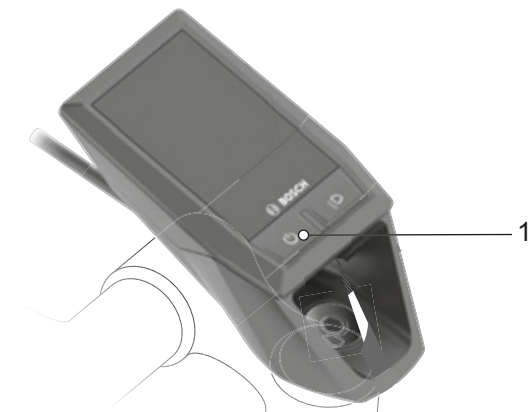
Figure 171: Position of On-Off button (control panel)
