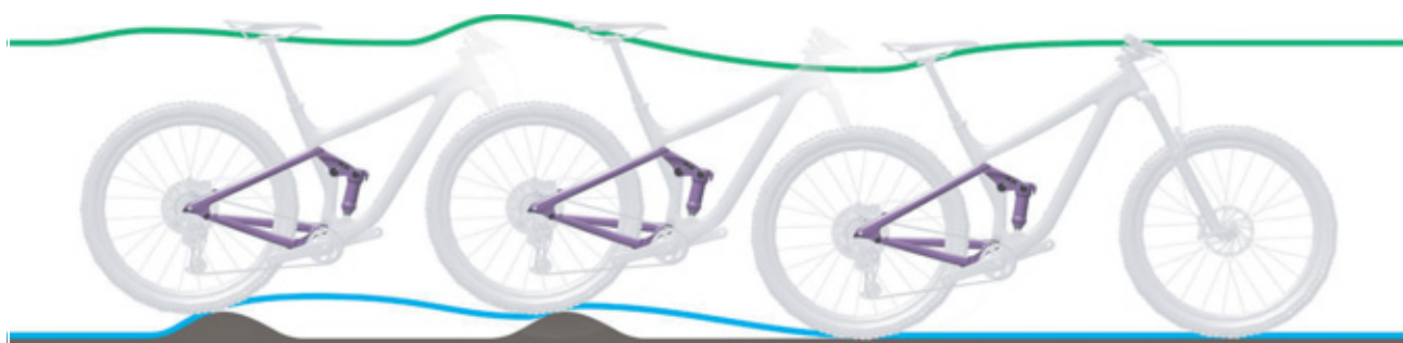
Figure 286: Rear frame damper rebounding too slowly
