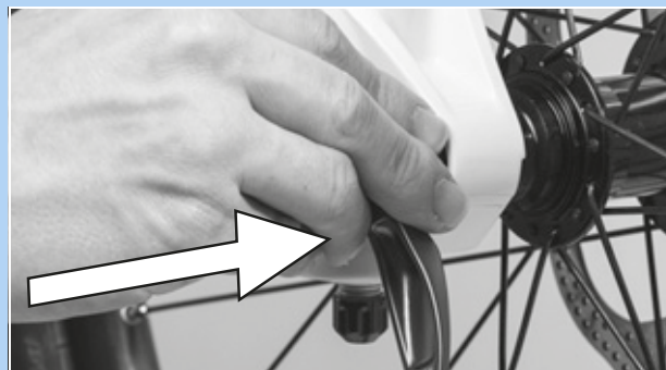
Figure 86: Inserting the quick release in the direction of the arrow
