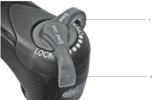
Figure 275: Changing compression adjuster to a softer setting
