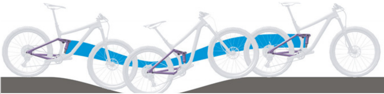
Figure 288: Excessively soft suspension in the rear frame damper on hilly terrain
