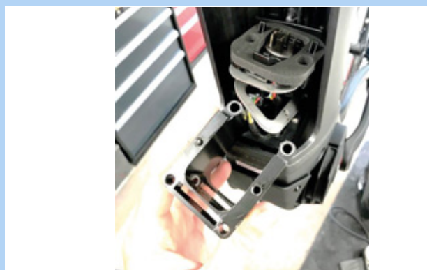
Figure 65: Pulling out the PowerTube adapter
