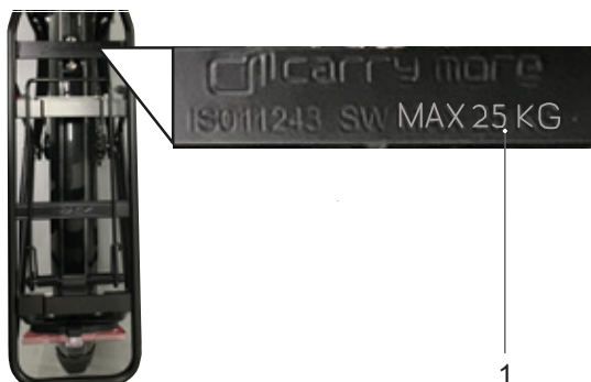
Figure 163: The maximum load bearing (1) capacity is indicated on the pannier rack.
