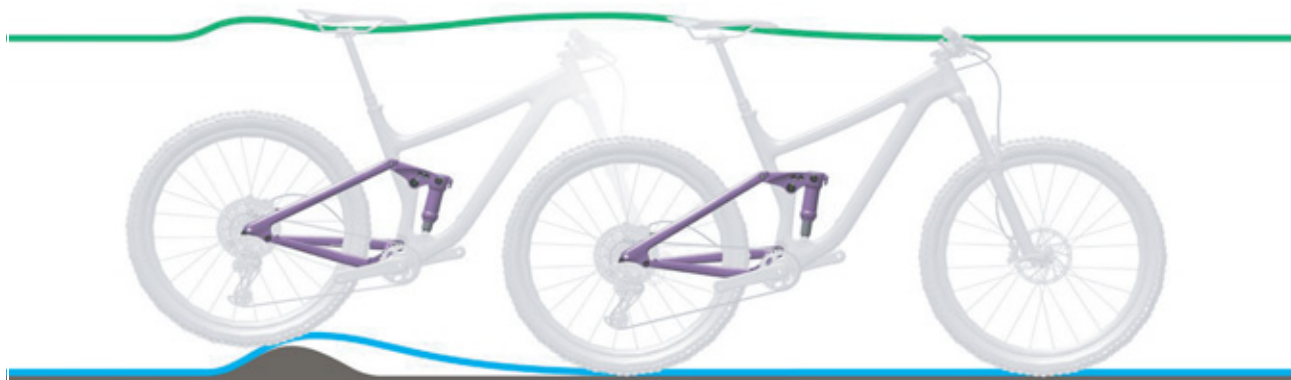
Figure 298: Excessively hard damping in the rear frame damper on bumps
