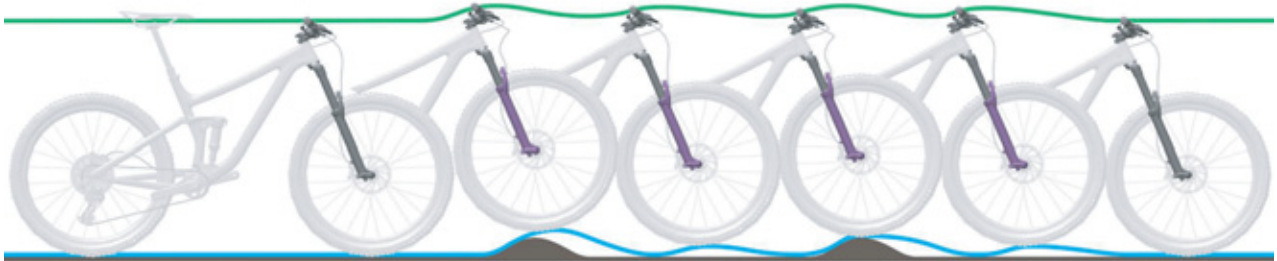
Figure 276: Suspension fork rebounding too quickly
