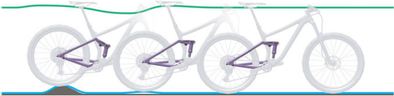
Figure 292: Rear frame damper rebounding too quickly
