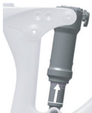
Figure 143: Moving the O-ring on the rear frame damper
