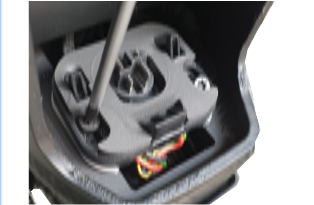
Figure 41: Undoing screws on battery mount
