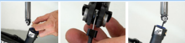
Figure 199: Attaching and pushing in the seat post
