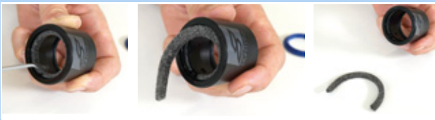
Figure 187: Removing the felt ring
