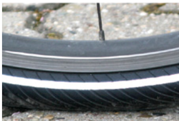
Figure 87: Correct tyre pressure. The tyre is barely deformed under the load of the body weight
