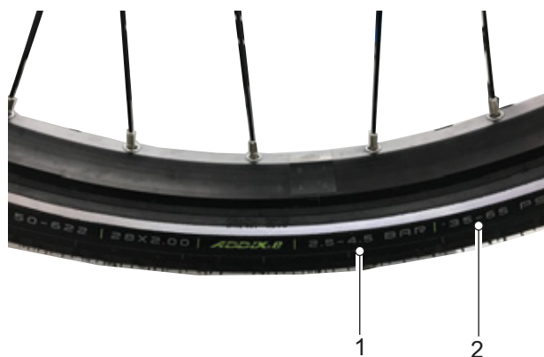
Figure 127: Tyre pressure in bar (1) and psi (2)
