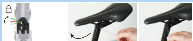
Figure 178: Closing the height adjustment
