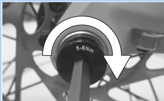
Figure 49: Tightening the securing screw
