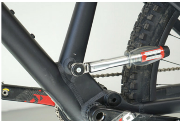
Figure 65: Tightening the seat post axle
