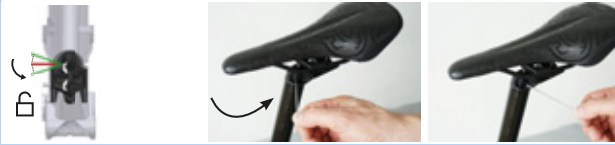
Figure 141: Moving height adjustment to the “Open position”
