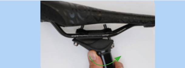
Figure 192: Opening the height adjustment
