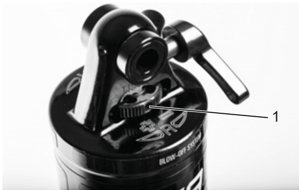
Figure 212: Suntour rebound adjuster wheel (1) on the rear frame damper
