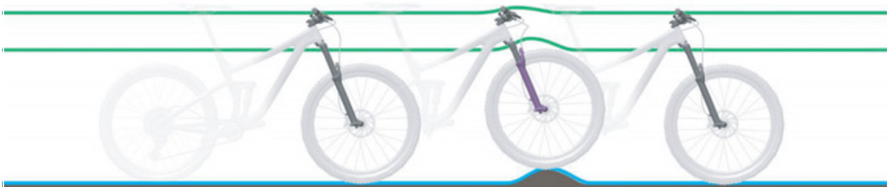
Figure 10: Optimum fork riding performance over bumps
