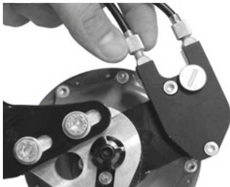
Figure 134: The tension adjuster on Rohloff hub versions with external switch control is located on the cable box positioned on the left-hand side
