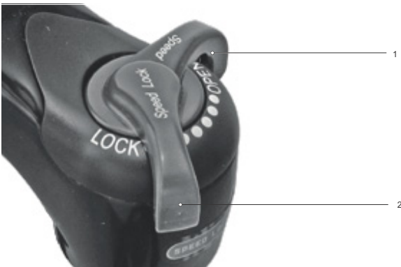
Figure 208: Changing compression adjuster to a harder setting
