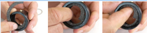
Figure 189: Inserting the felt ring
