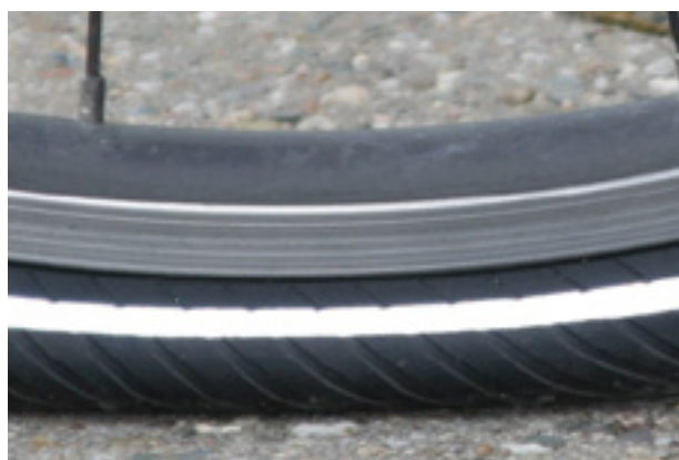
Figure 88: Much too little tyre pressure
