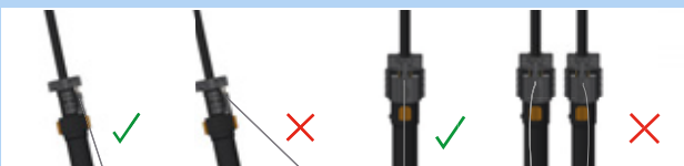
Figure 168: Correct and incorrect Bowden cable
