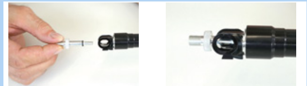
Figure 158: Screwing the valve adapter in
