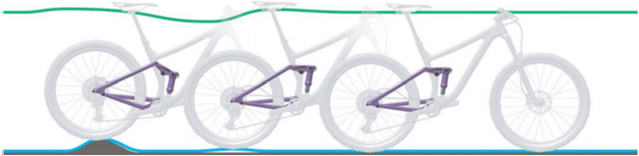
Figure 211: Rear frame damper rebounding too quickly
