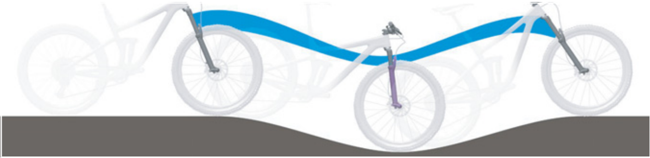
Figure 207: Excessively soft suspension in the suspension fork on hilly terrain
