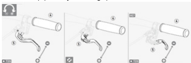
Figure 63: Adjusting the grip distance on a Magura disc brake lever
