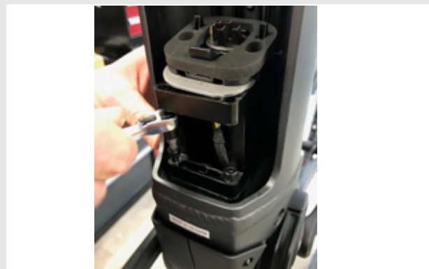
Figure 24: Removing the 4 mm hexagon screws
