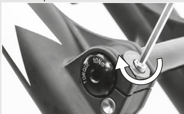
Figure 41: Tightening the securing clip
