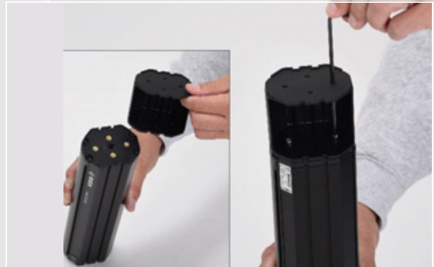
Figure 33: Fitting the PowerTube extension
