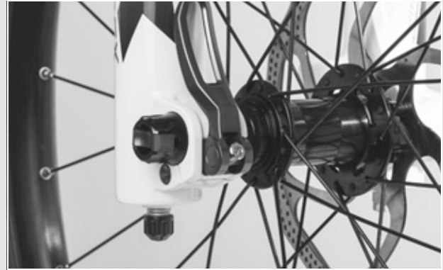
Figure 46: Perfect position for the clamping lever
