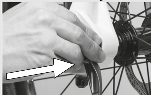
Figure 49: Pushing the quick release in
