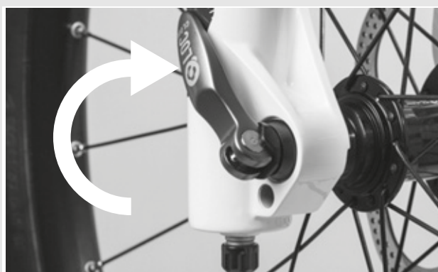
Figure 51: Closing the quick release
