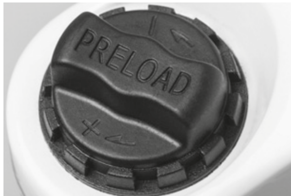
Figure 65: Sag setting wheel on the suspension fork crown
