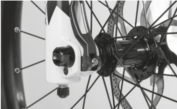
Figure 91: Adjusting the quick release clamping force
