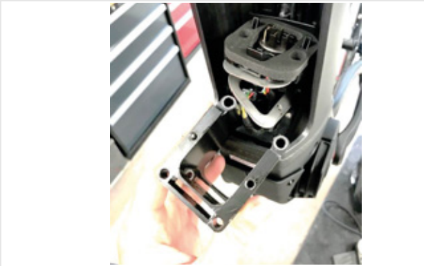
Figure 26: Pulling out the PowerTube adapter
