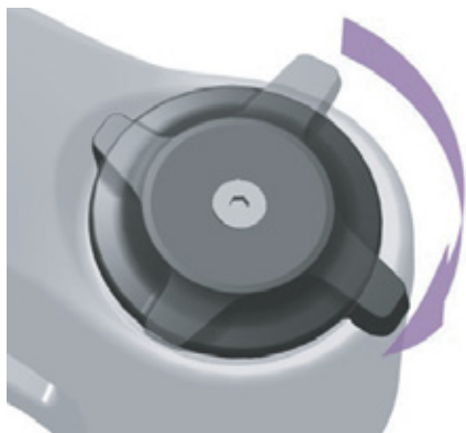
Figure 98: Changing compression adjuster to a harder setting
