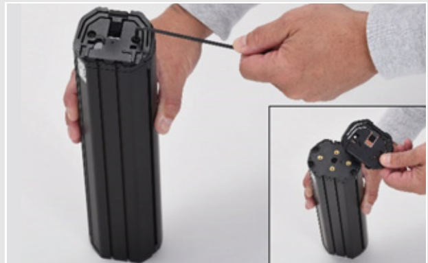
Figure 29: Detaching the upper interface
