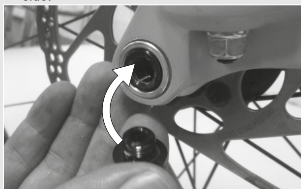
Figure 38: Pushing the quick release lever into the axle
