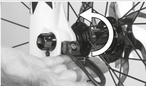
Figure 45: Securing the lever
