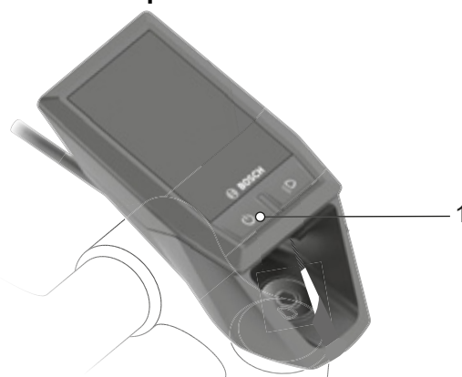
Figure 77: Position of On-Off button (on-board computer)
