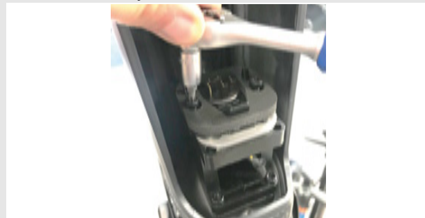
Figure 23: Undoing screws on battery mount
