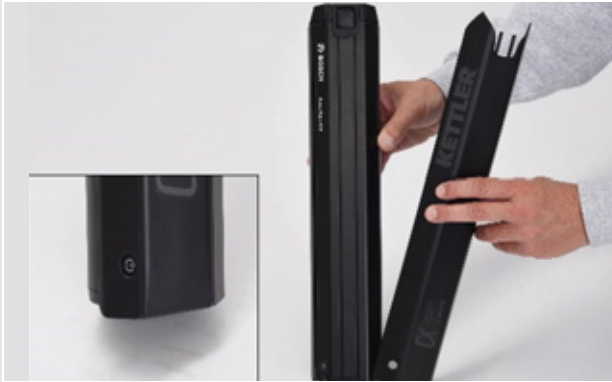
Figure 31: Pushing the battery cover onto battery
