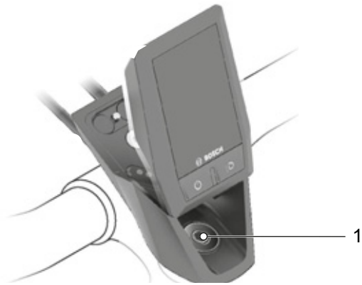
Figure 75: Position of headset screw
