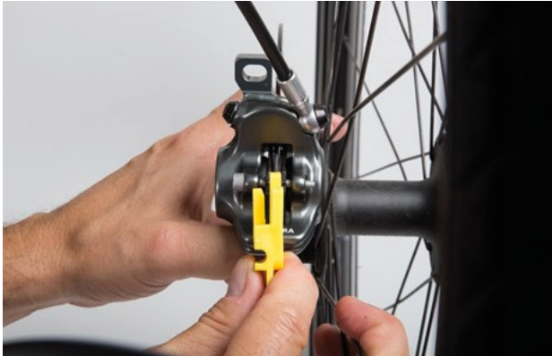
Figure 120: Checking the brake lining when fitted with the help of the transport safety wear gauge
