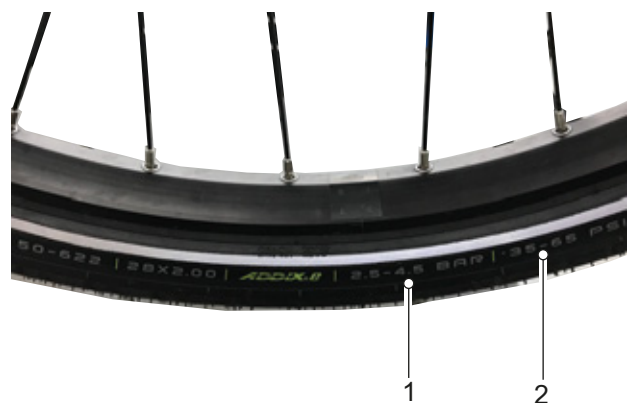
Figure 117: Tyre pressure in bar (1) and psi (2)
