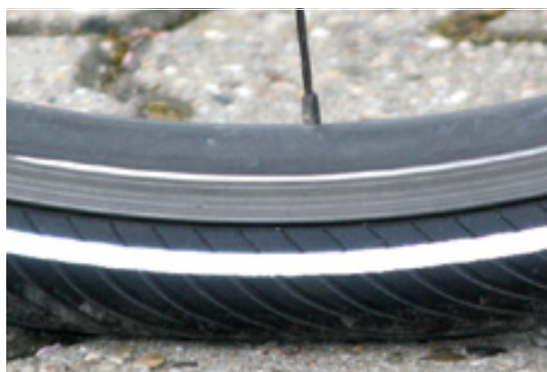
Figure 79: Correct tyre pressure. The tyre is barely deformed under the load of the body weight
